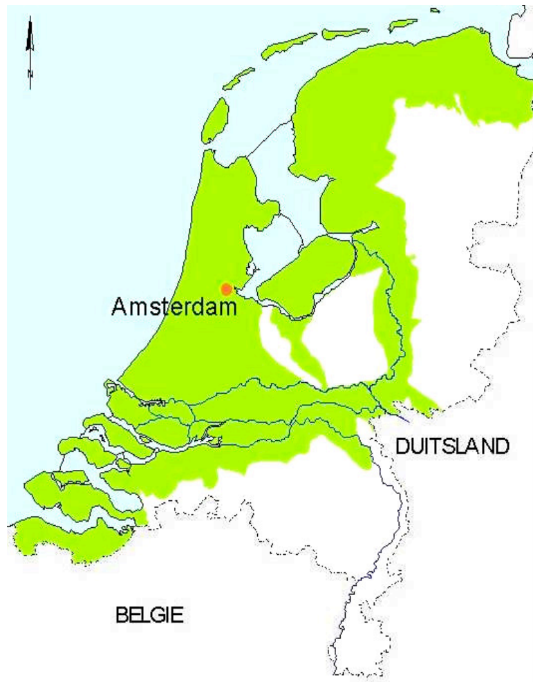
Figure 3 Dutch delta, the part of The Netherlands that would be flooded without dikes (Source: rijkswaterstaat.nl).
